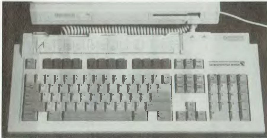
Figure 1. The keyboard is similar to that of an IBM AT — the red function keys are a remnant of the old BBC Model B. Note the adjustable plastic prompt card window, which contains a replaceable, application specific card.
