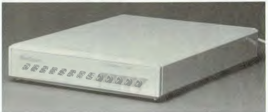
Figure 2. The NetComm Smart Modem 1234SA adds autoranging, synchronous communications and software to the features of the 1234.
