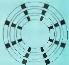
Figure 1* Perfectly aligned tracks. The black areas are "read only." These store critical track and sector ID information. The white areas are data sectors and store your system, programs and data.
