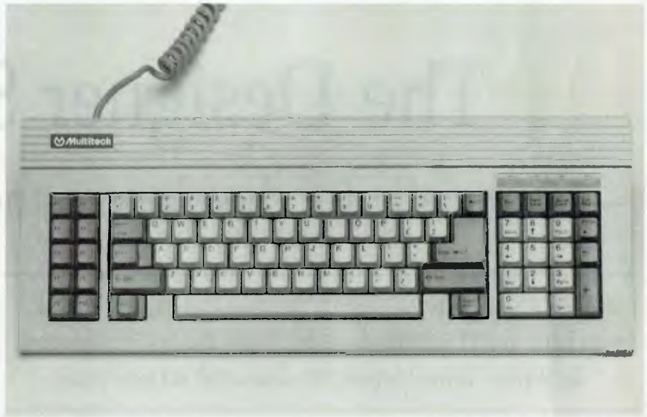
Figure 1. The Acer's AT-style keyboard has excellent audio and tactile feedback — and it plugs into the front of the system box. Indicators for Caps, Num and Scroll Lock, and Power can be seen above the keypad.
